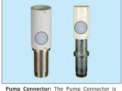
fabricated assembly of stainless steel pipe / cast iron having one end threaded to match the socket threads of the pump and the other end to match with the Jain Thread Loc Plus coupler
